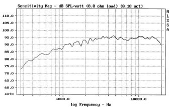
Driver was mounted rigidly on an IEC baffle. Microphone distance is 0.5m, input voltage 2.83VRMS and normalized to 1m. 1/12 octave smoothing was applied.
