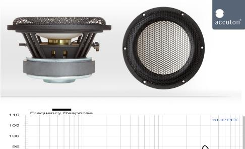
MAIN FEATURES : OVERHUNG MOTOR DESIGN 38 MM TITANIUM VC FORMER SOFT HIGHSHAPE RUBBER SURROUND VENTED VC, POLE PIECE & SPIDER 35 HZ - 2.5 KHZ IN VENTED BOX
