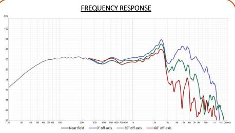
Note: The frequency responses above show SPL in 0° (blue), 30° (green) and 60° (red) angle mounted on a  $1.66 \times 1.35$  m baffle in free air. Microphone at 0.5 m, SPL normalized to 1 m and input at  $2.83 \text{ V}_{RMS}$ . Nearfield response (black) below 250 Hz. Impulse response limited to 4 ms and 1/24 smoothing applied.
