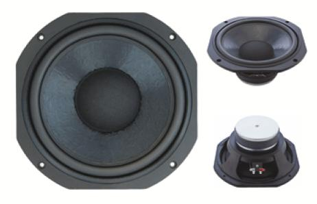
The B250.8 features a symmetrical field magnet and long voice coil for large linear excursion capability. It also has double rear suspensions whose characteristics are matched to that of the motor assembly for stability and linearity at high drive levels. An extended centre pole is utilised to minimise distortion inducing inductance swing at high power levels. The Thiele-Small parameters are optimised for bass extension.
