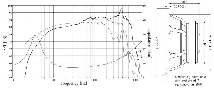
The frequency responses above show measured free fields ound pressure in 0, 30, and 60 degrees angle using a 12L closed box. Input 2.83 VRMS, microphone distance 0.5m, normalized to SPL 1m.The dotted line is a calculated response in infinite baffle based on the parameters given for this specific driver. The impedance is measured in free air without baffle using a 2V sine signal.
