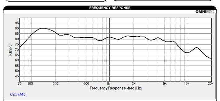
1/3<sup>rd</sup> octave smoothing - measurement taken with transducer adhered off-center on a 12" x 12" x 1/2" foam core board in an infinite baffle setup.
