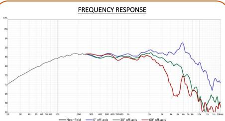
Note: The frequency responses above show SPL in 0° (blue), 30° (green) and 60° (red) angle mounted on a 1.66 x 1.35 m baffle in free air. Microphone at 0.5 m, SPL normalized to 1 m and input at 2.83  $V_{\text{RMS}}$ . Nearfield response (black) below 250 Hz. Impulse response limited to 4 ms and 1/24 smoothing applied.
