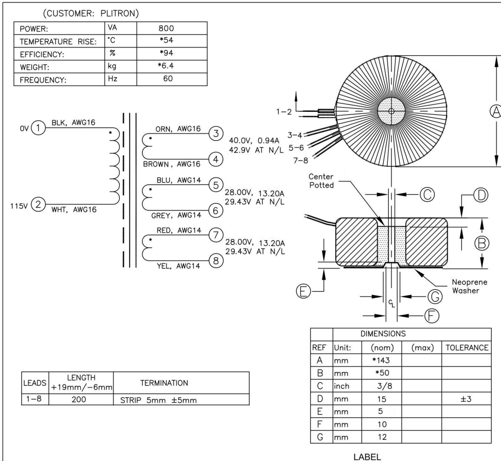
PLITRON MANUFACTURING INC. 8831 - XO-O4 DATE CODE F: 60Hz
