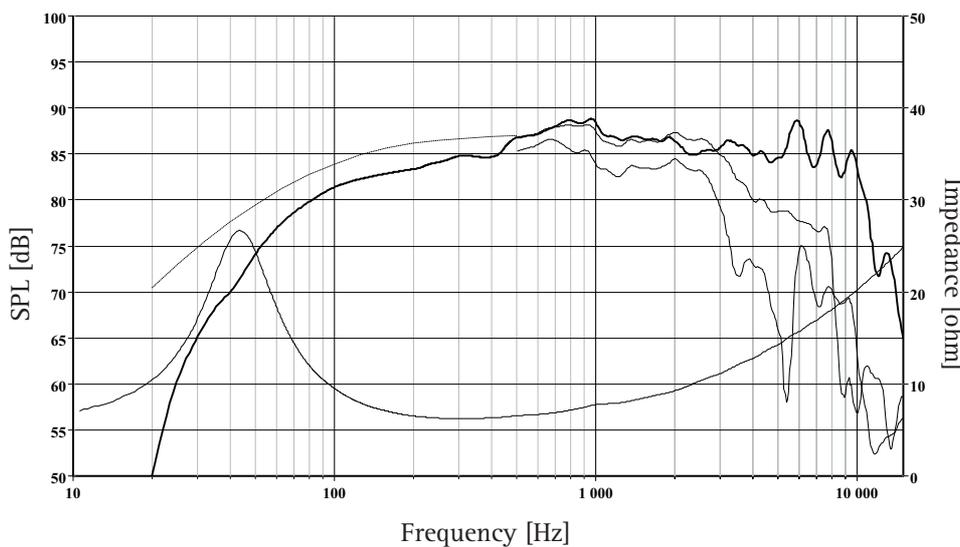
The frequency responses above show measured free field sound pressure in 0, 30, and 60 degrees angle using a 7L closed box. Input 2.83 V<sub>RMS</sub>, microphone distance 0.5m, normalized to SPL 1m. The dotted line is a calculated response in infinite baffle based on the parameters given for this specific driver. The impedance is measured in free air without baffle using a 2V sine signal.
