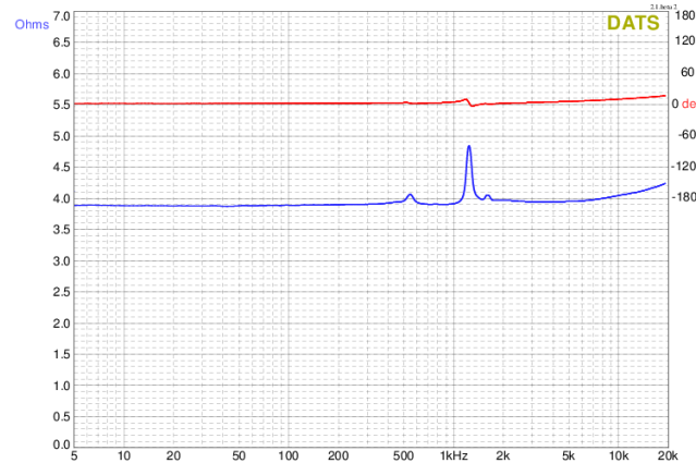
Measurement taken with transducer uncoupled facing upward.
